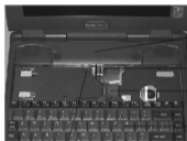
Keyboard top cover PJ11 Keyboard cable Keyboard
